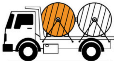
Secure drums adequately before transportation.
